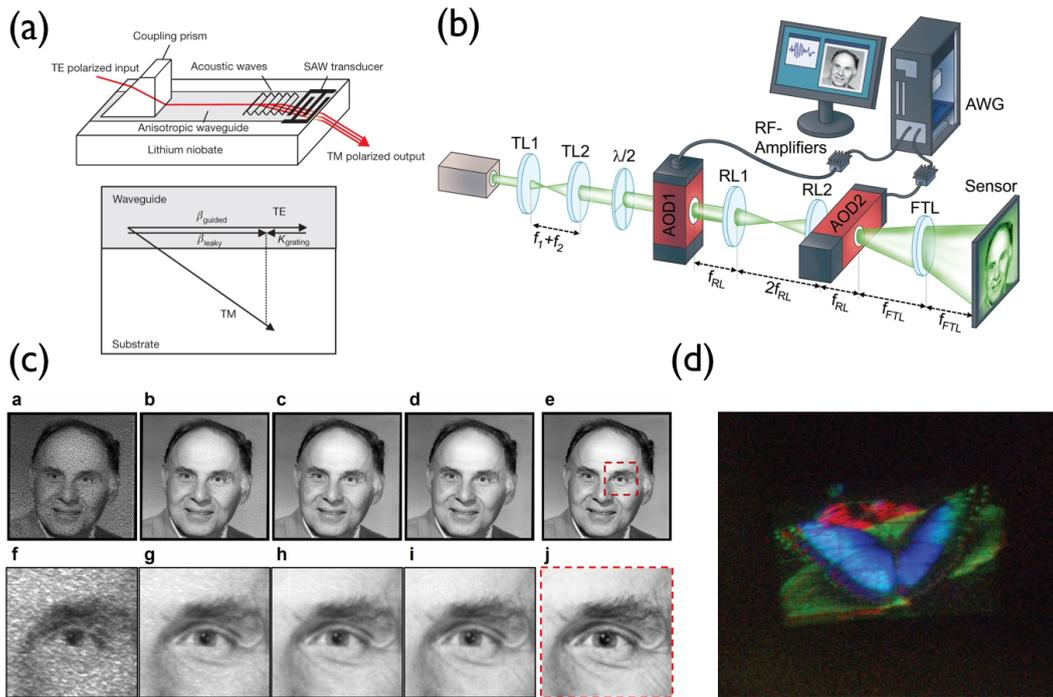
Fig. 1.5: a) Schematics of the side and top view of a waveguide based acousto-optic spatial light modulator. b) Schematic of a free space acousto-optic holographic projector. c) Measured holographic projections at various detector integration time employing the device from b). d) Observed holographic projection employing a device structure similar to a). Multicolors were achieved through wavelength superpositioning. Images adapted from [75, 76, 77].
