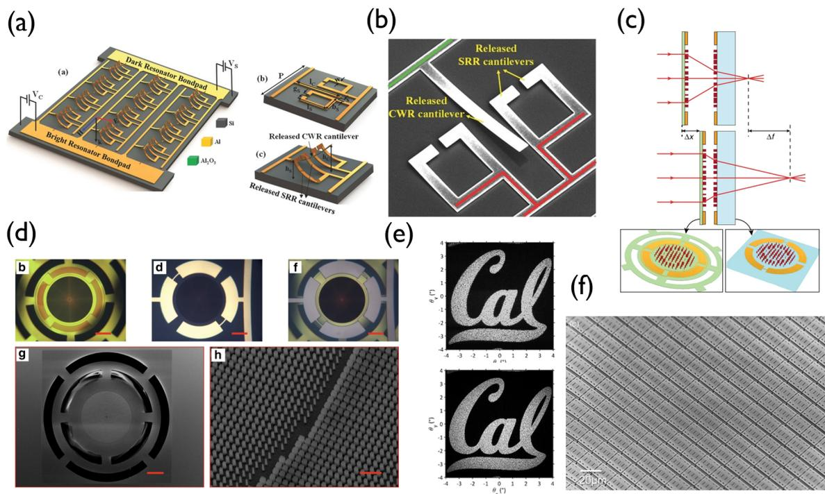
Fig. 1.7: a) Artists impression of a split ring resonator actuated by electrostatic MEMS. b) SEM image of a single unit cell of the device in a). c) Schematic of a doublet metasurface built on a MEMS actuator to provide tunability. d) Microscope and SEM images of the doublet metasurface constituents shown in c) e) Simulated and measured holographic projection from a grating metasurface actuated by MEMS. f) SEM image of MEMS actuated gratings used in e). Images adapted from [114, 115, 116].
